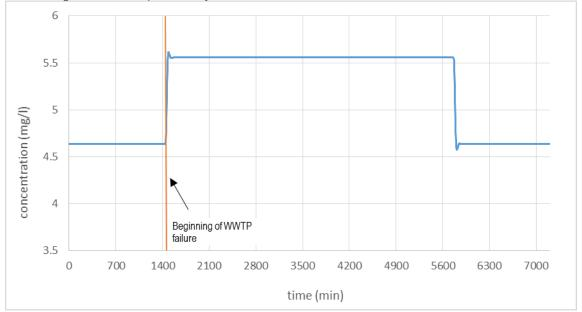
Figure 6 Change in BOD₅ concentration at 53 + 360 rkm in the period between January 14, 2015 (11:59 p.m.) and January 19, 2015 (11:59 p.m.)
