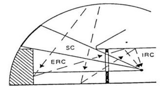
Figure 1 Daylight factor [4]
