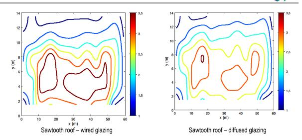
Figure 5 Plot of daylighting factor
