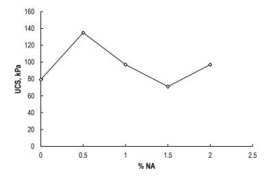
Figure 5 Determination of the Optimal NA Content
