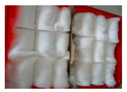
Figure 2 Specimens Subjected to Wetting Cycle for 24 hours
