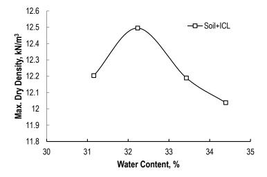
Figure 4 Compaction Curve for ICL-Stabilized Soil Sample
