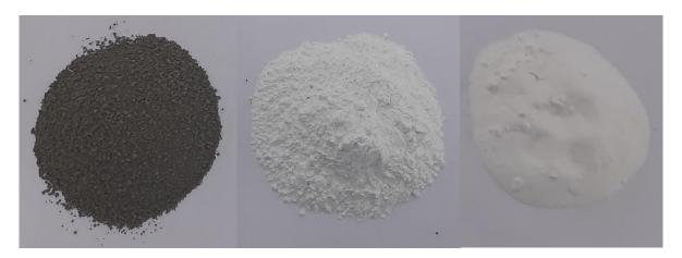
Figure 1 Materials Used: Soil, Lime, and NA (In the Order of Appearance)
