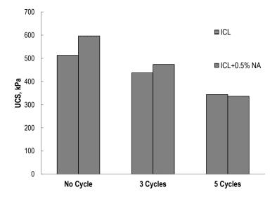
Figure 9 Durability of NA-Amended Lime-Stabilized Soil Samples
