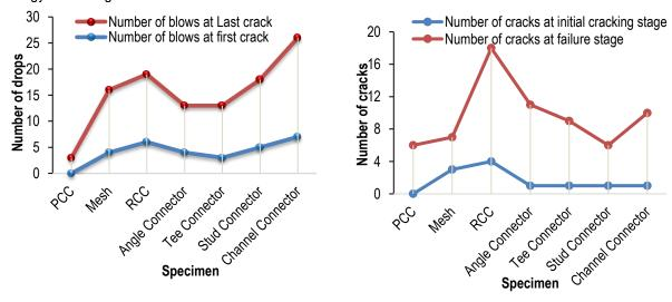
Figure 9 Comparison between the number of drops and number of cracks with slab specimens
