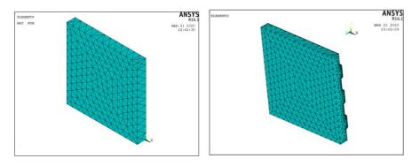
Figure 11 Mesh model of plain concrete slab and steel-concrete composite slab
