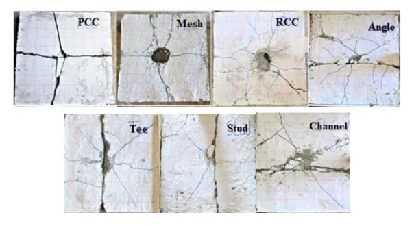
Figure 8 Ultimate failure of the M30 grade slab specimens
