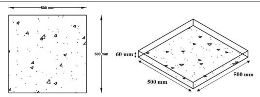
Figure 2 Dimensions of the specimen
