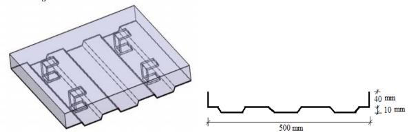
Figure 1 Details of steel decking sheet
