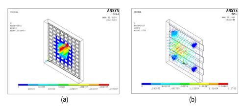
Figure 13 Vector plot of the mesh slab and composite slab
