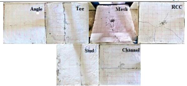
Figure 7 Initial crack of the M30 grade slab specimens
