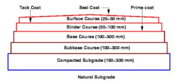
Figure 1 Pavement structure
