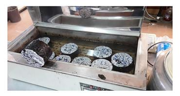
Figure 5 Putting samples in the water bath
