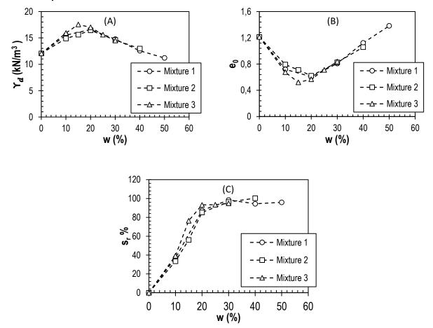
Figure 2 Variation of dry unit weight (A), initial void ratio (B) and degree of saturation (C) against the water content
