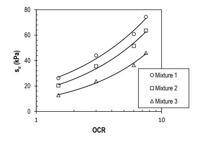
Figure 8 Evolution of undrained shear strength against OCR
