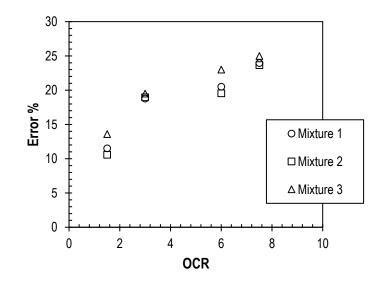
Figure 10 Error related to the prediction of  $\sigma'_{\rm p}$  with respect to the overconsolidation ratio
