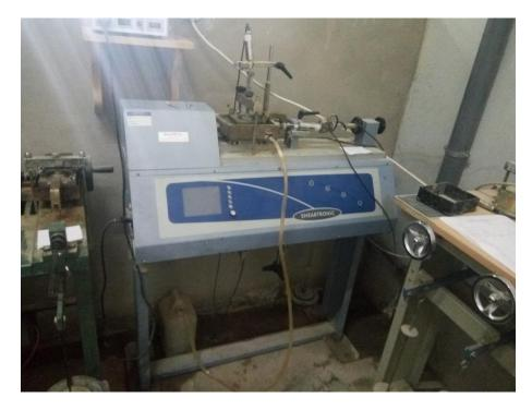
Figure 5 Direct-shear test apparatus
