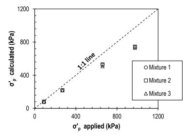
Figure 9 Comparison between calculated and applied values of  $\sigma^\prime{}_p$  for the three mixtures
