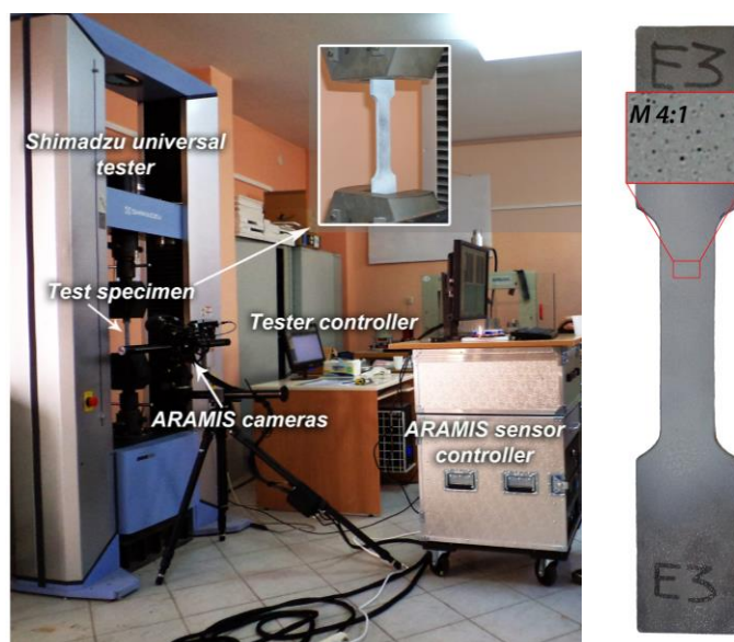
Figure 5 Test setup along with applied stochastic color-spray pattern on test specimen E3
