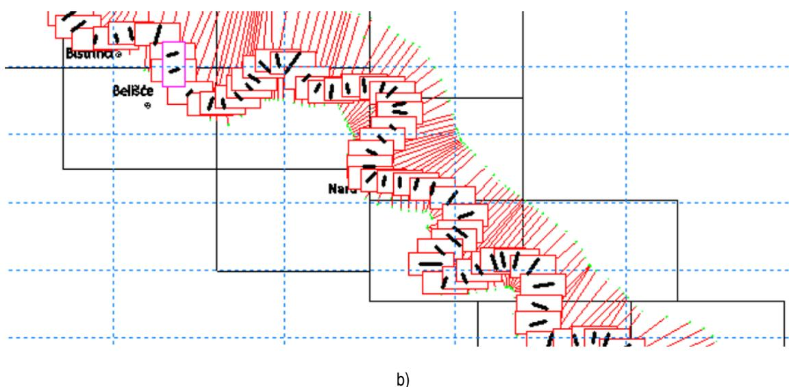
**Figure 2** Ground plan of the modeled reach of the Drava River, with the locations of the defined cross-sections in the MIKE 11 software package (a) and Detail of the modeled reach of the Drava River with the locations of the defined cross-sections in the MIKE 11 software package (b)
