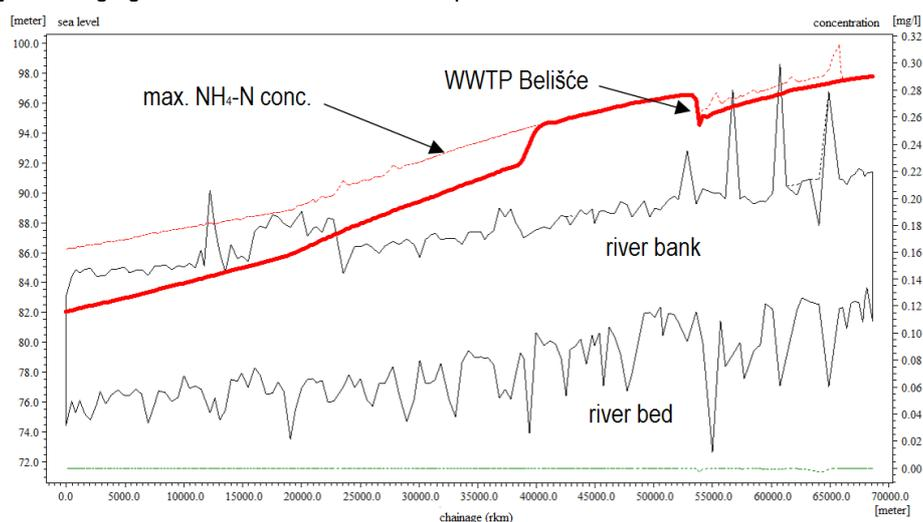
**Figure 7 Spatial distribution of ammonia nitrogen concentration (NH<sub>3</sub>-N) (mg/l) after the Belišće WWTP failure**
