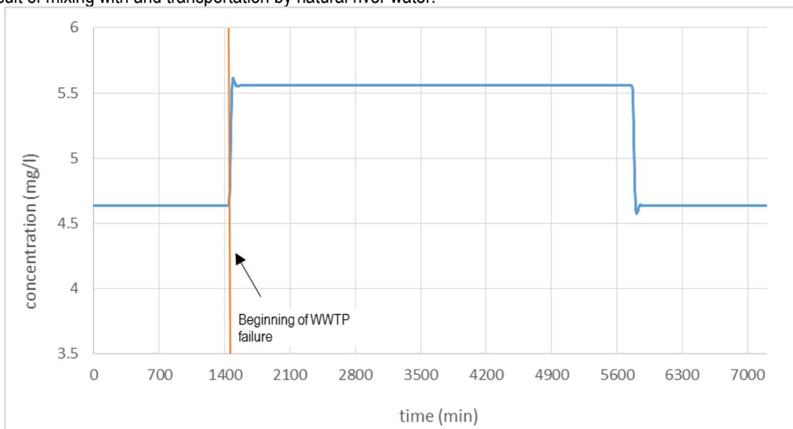
**Figure 6 Change in BOD<sub>5</sub> concentration at 53 + 360 rkm in the period between January 14, 2015 (11:59 p.m.) and January 19, 2015 (11:59 p.m.)**
