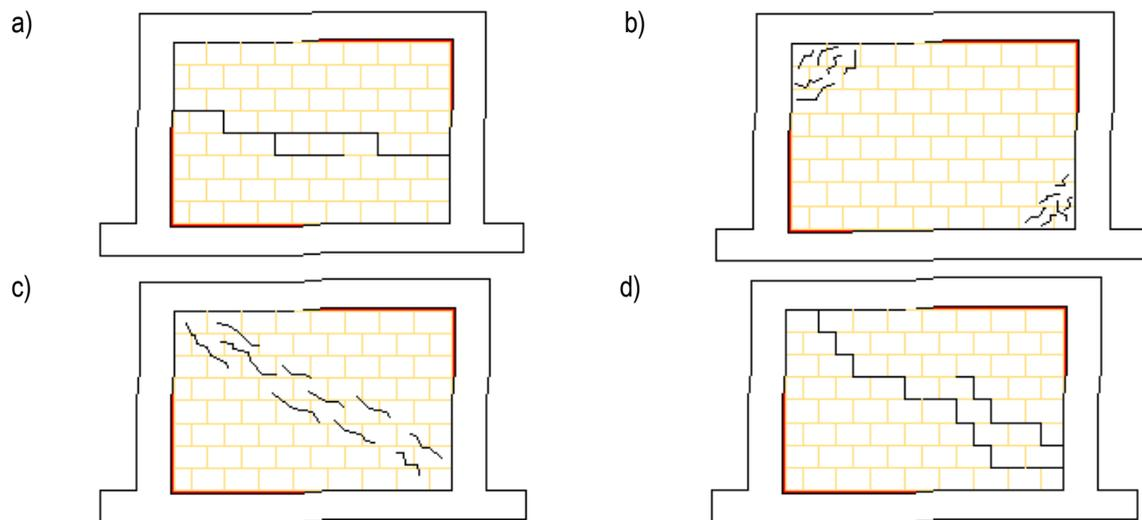
**Figure 1. Equivalent strut, showing the modes of failure for the infill:**
