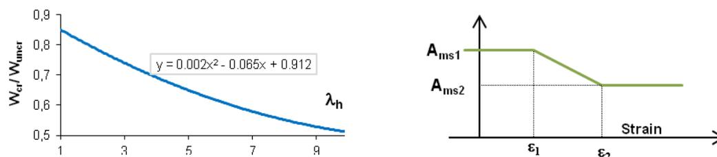
**Figure 4. a) Ratio of strut width between cracked and uncracked masonry infills[19]
