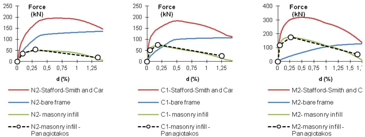
**Figure 8. Local response of masonry infill, comparing numerical results and calculated curve, by Panagiotakos [26]**
