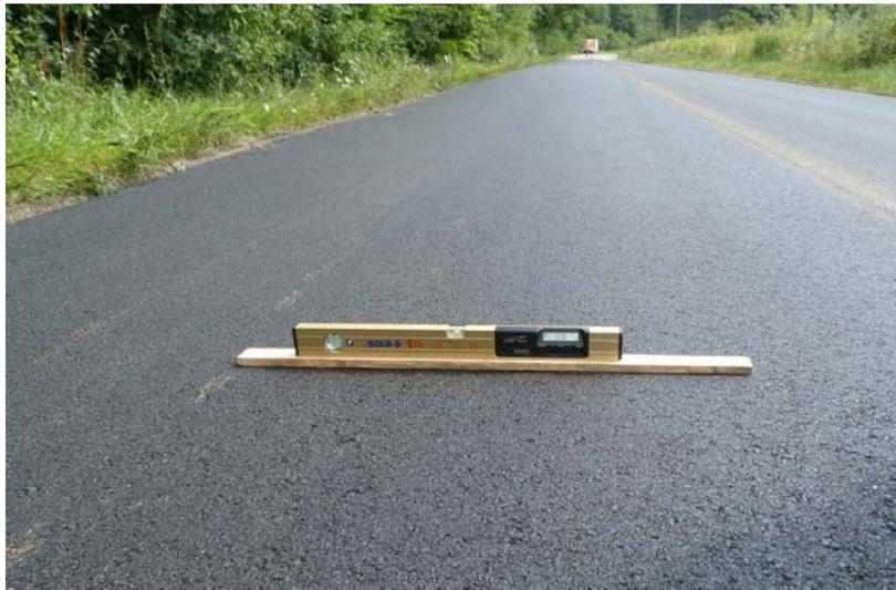
Figure 4. Inclinometer on new layer
