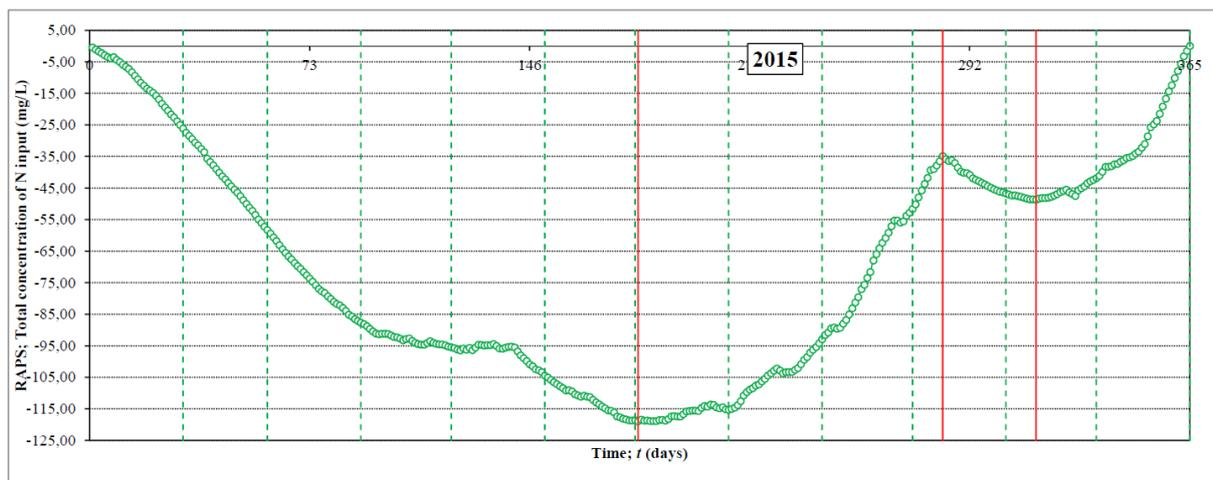
**Figure 3 Application of the RAPS method for the input values of total daily nitrogen in 2015 at the Čakovec wastewater treatment plant**
