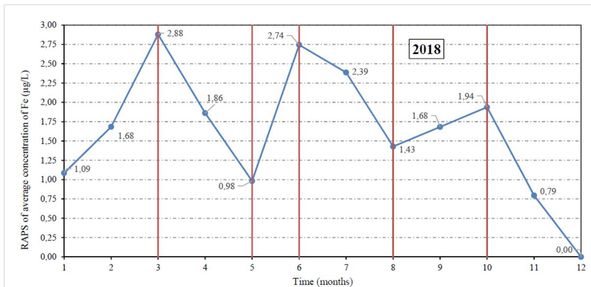
**Figure 6 Application of RAPS method for an average monthly concentration of Fe (µg/L) values in 2018 for the Osijek water supply system**
