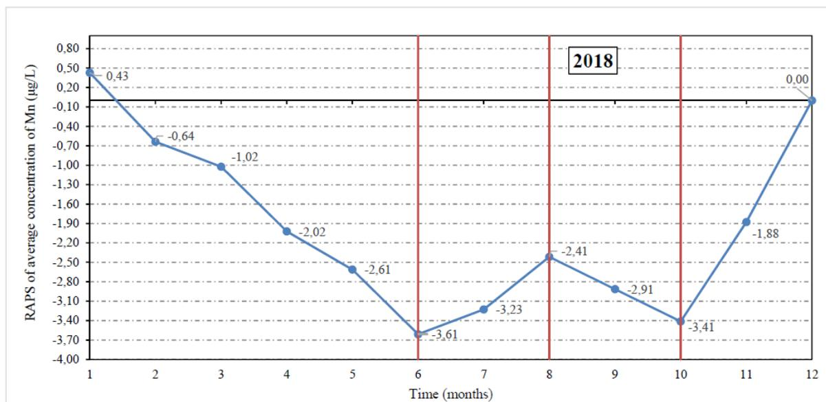
**Figure 8 Application of the RAPS method for an average monthly concentration of Mn (µg/L) values in 2018 for the Osijek water supply system**
