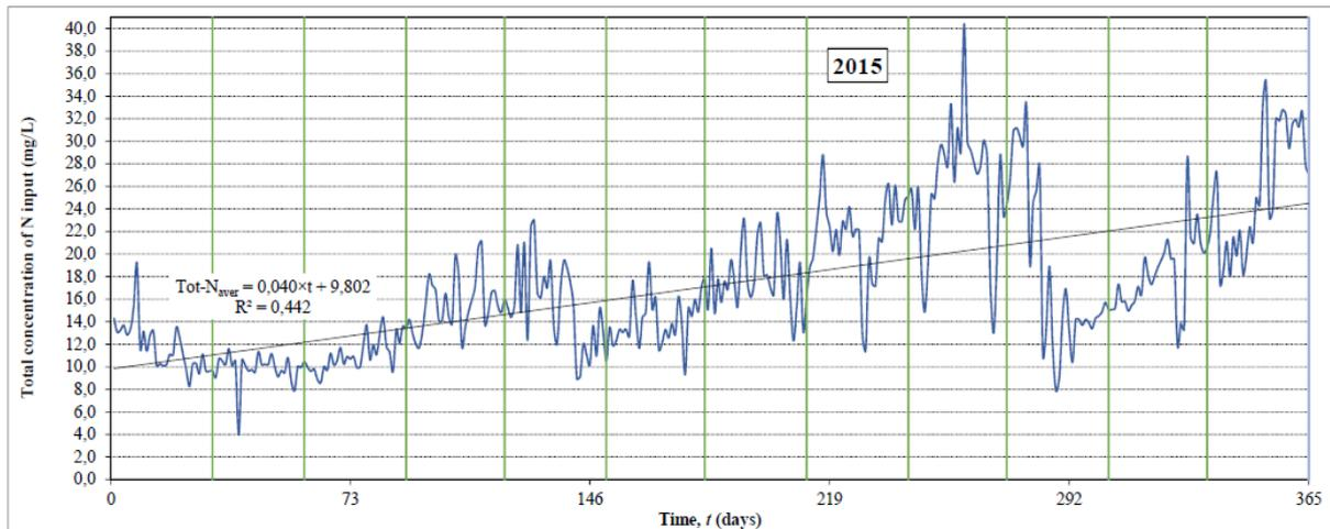
**Figure 2 Linear trend of the input values of total daily nitrogen in 2015 at the Čakovec wastewater treatment plant**
