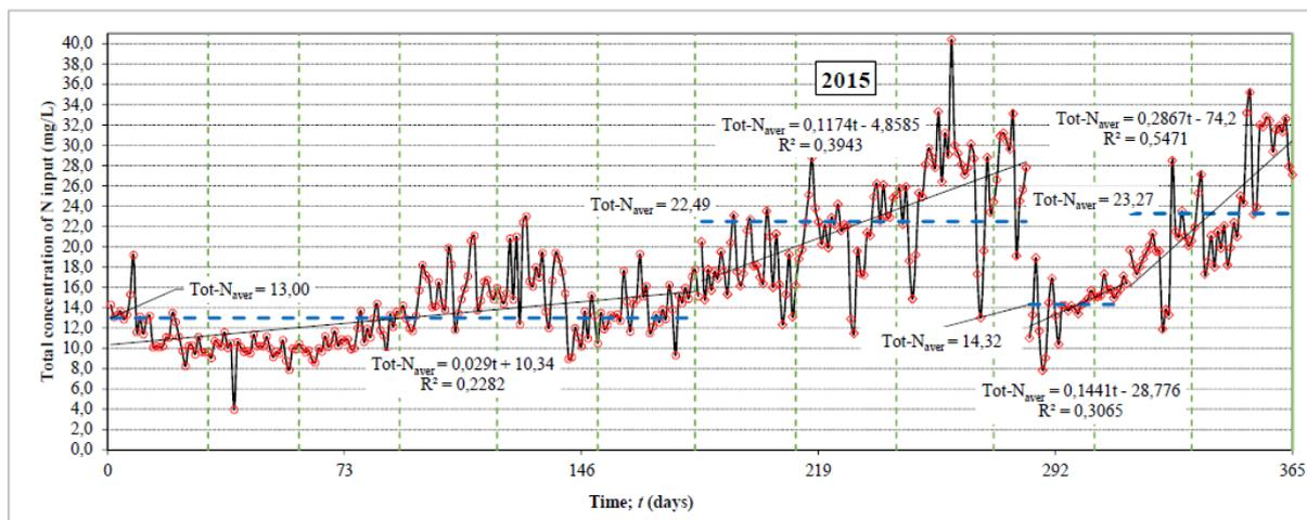
**Figure 4 Application of RAPS method for the input values of total daily nitrogen in 2015 at the Čakovec wastewater treatment plant**
