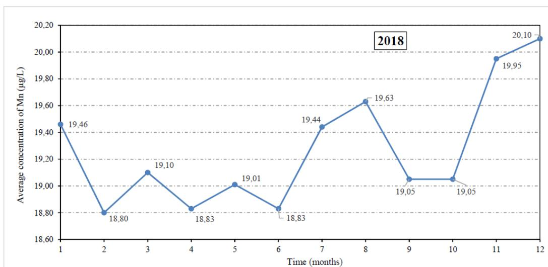
**Figure 7 Input values of an average monthly concentration of Mn (µg/L) values in 2018 for the Osijek water supply system**
