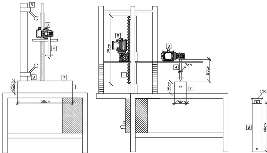
Figure 4 Test machine design drawings
