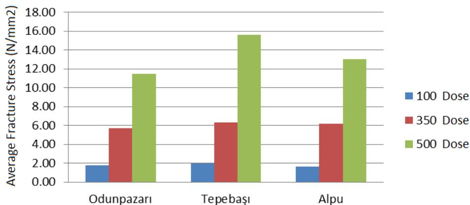
**Figure 6 Effect of cement dosage**
