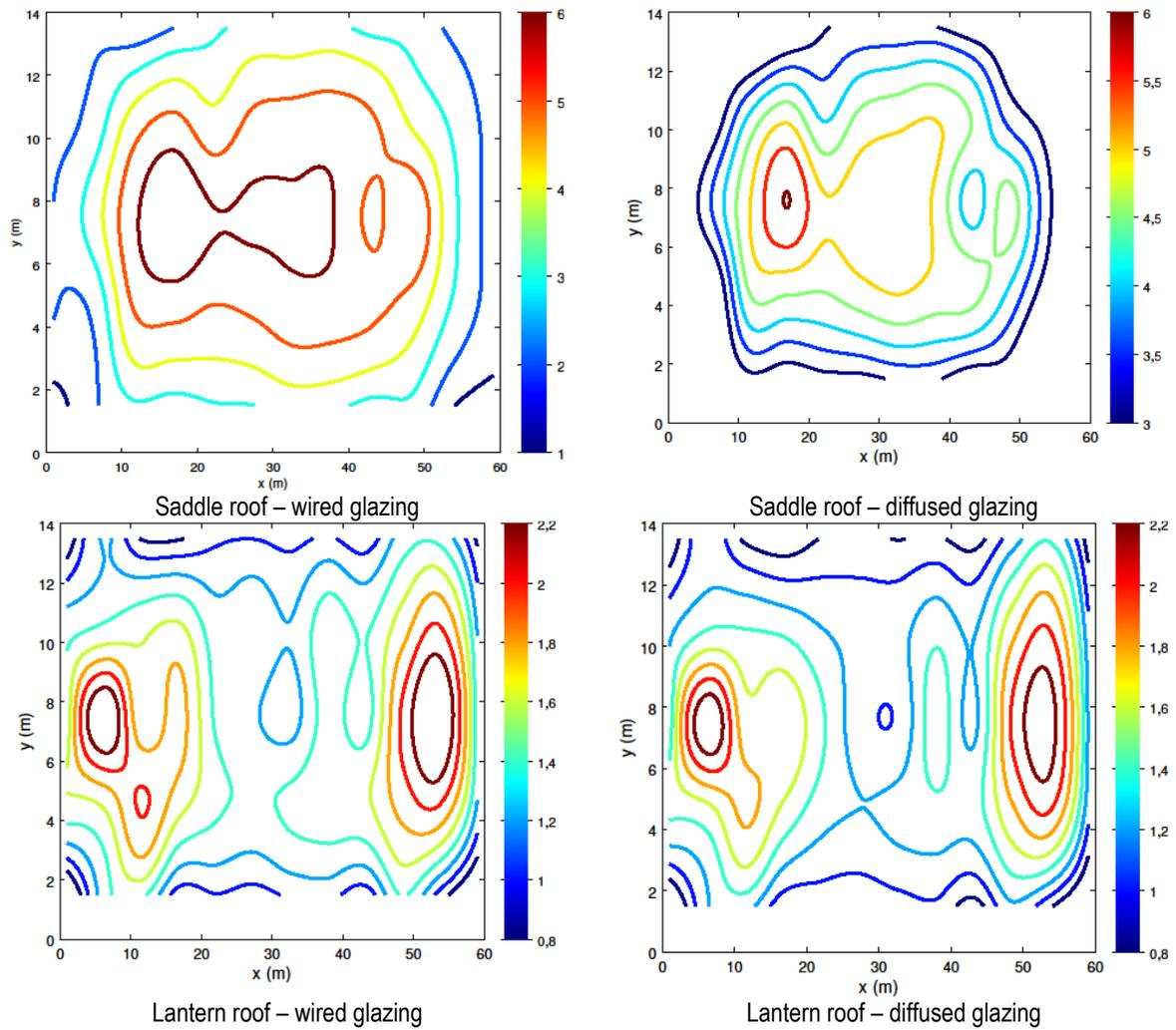
Figure 4 Plot of daylight factor
