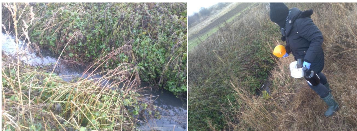
Figure 1 Peripheral canal of the landfill site L and process of collecting leachate samples
