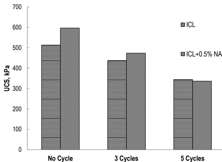
Figure 9 Durability of NA-Amended Lime-Stabilized Soil Samples
