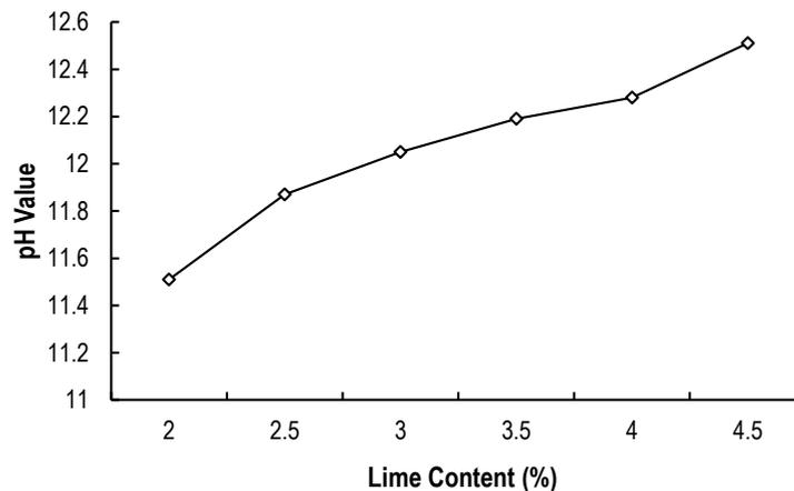
Figure 3 Eades and Grim pH Test for the ICL Determination
