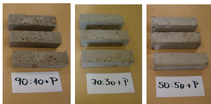
Figure 3 Samples with EWPA after 28 days of curing
