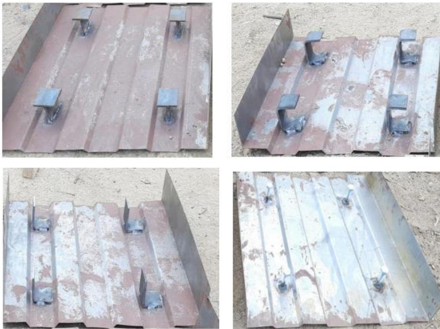
**Figure 3 Steel decking sheet with welded shear connectors**
