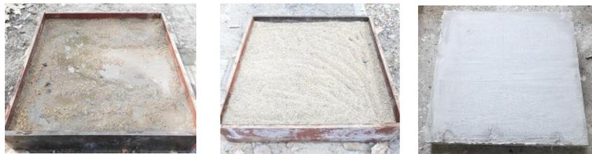
**Figure 5 Preparation stages of specimens**
