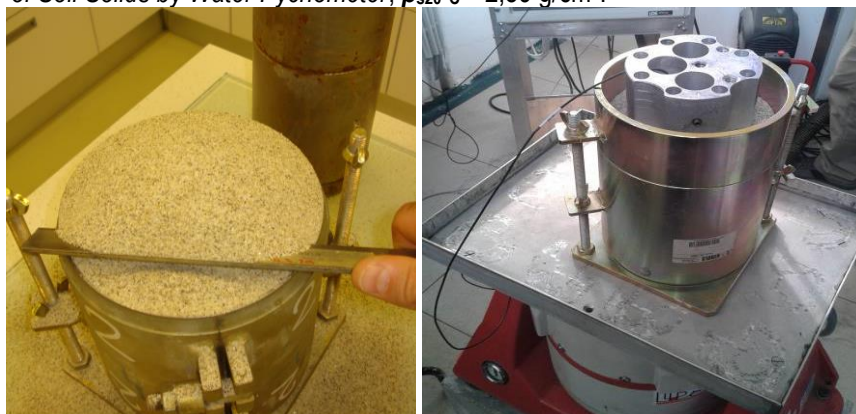
Figure 1 Testing of minimum (left) and maximum (right) index densities of sand
