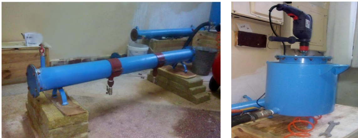
Figure 6 Laboratory test bench and mortar pumping machine
