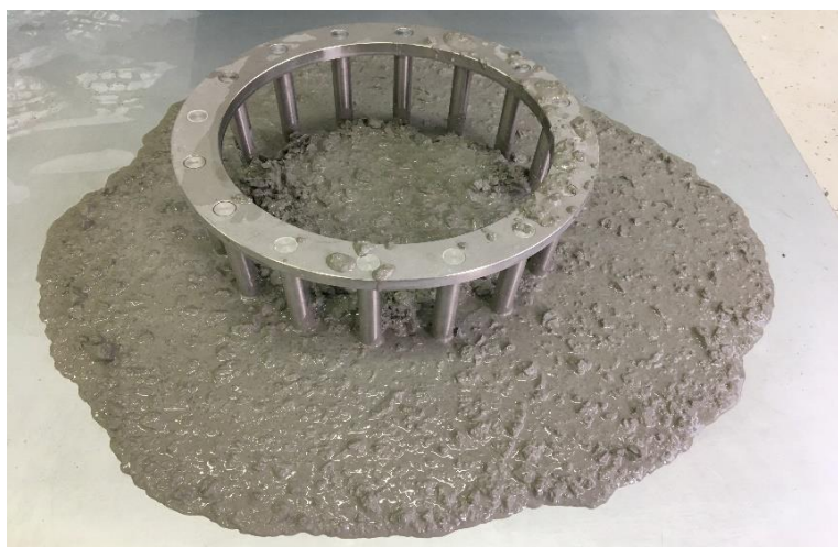
Figure 4 Testing of mixture M17 by J-ring method [22]
