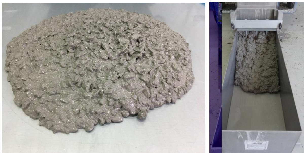
Figure 3 Mixture M10 (slump-flow) [22] and M1 (L-box) [21]
