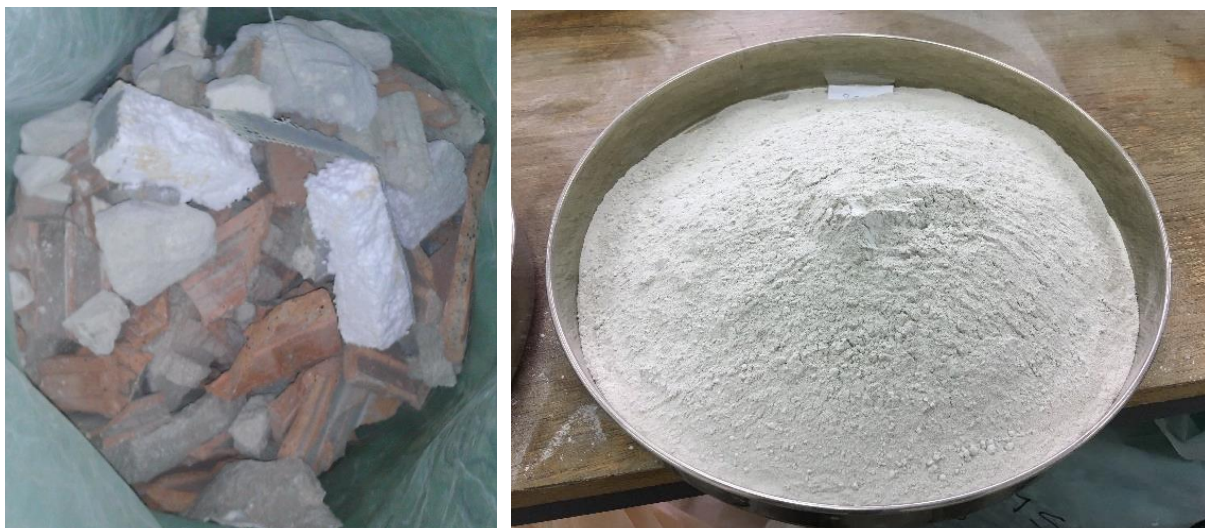
Figure 2 Material for preparation of filler F1 (left) [21] and F32 — fraction 0.063–0.125 mm (right) [22]
