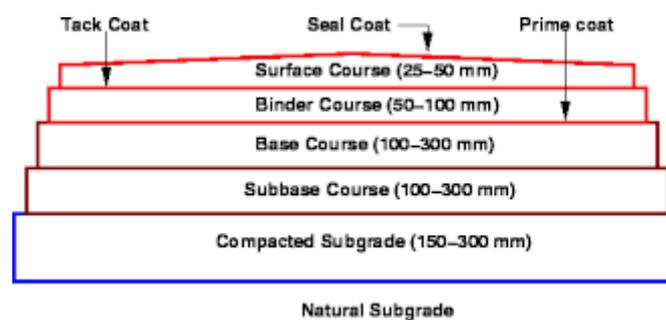
Figure 1 Pavement structure
